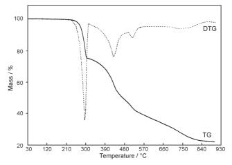
Fig. 1 TG-DTG curves of [Tb<sub>2</sub>(o-MBA)<sub>6</sub>(PHEN)<sub>2</sub>] using a heating rate of 5°C min<sup>-1</sup>
